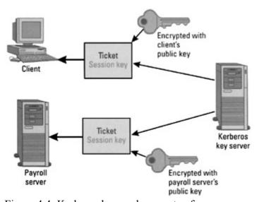
Figure 4.4: Kerberos key exchange, step four.
