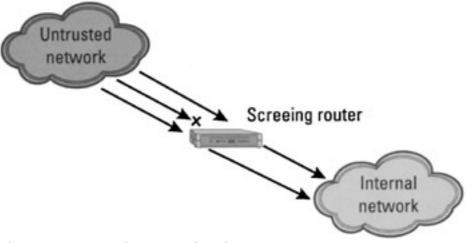
Figure 12.2: Screening router function.
