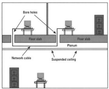
Figure 9.3: Plenum cable.
