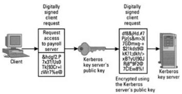
Figure 4.3: Kerberos key exchange, step three.
