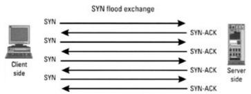
Figure 2.7: SYN flooding exchange.
