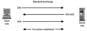
Figure 2.6: Normal TCP/IP handshake.
