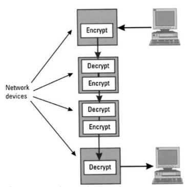
Figure 11.1: Node-to-node encryption.
