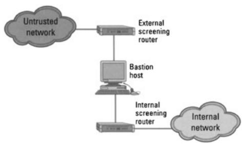
Figure 12.7: Screened subnet configuration.
