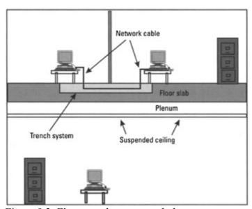
Figure 9.2: Floor trench system and plenum.
