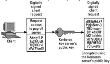
Figure 4.2: Kerberos key exchange, step two.
