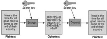
Figure 3.3: Symmetric key encryption.
