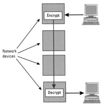
Figure 11.2: End-to-end encryption.
