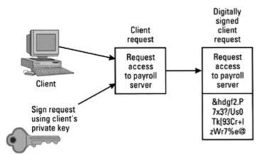
Figure 4.1: Kerberos key exchange, step one.
