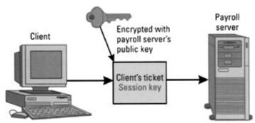
Figure 4.5: Kerberos key exchange, step five.
